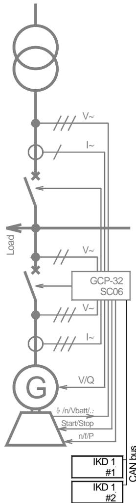
The digital inputs are read by the IKD 1 and transferred via the CAN bus to the control unit (incl. alarm class). Each alarm input may have a delay as well as the control logic (NO/NC) configured individually during set up. The status of the alarm input is monitored in the control device and will show the alarm text in its display. The alarm class assigned in the control device evaluates the alarm input and reacts accordingly.
